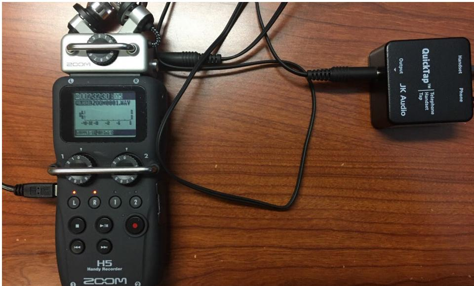
3. Connect the 1/8" (3.5mm) Mono Audio cord (supplied by JK Audio) to the "Output" jack of the QuickTap and to the "Line In" jack of the Zoom H5 capsule.
