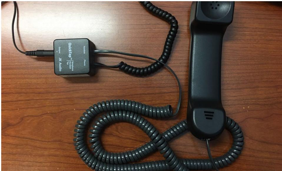
5. Connect a handset coiled cord the handset, then connect the opposite end to the "Handset" jack on the QuickTap.
