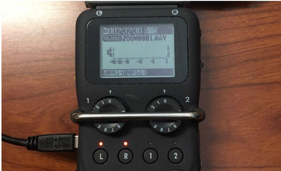
2. For the Zoom H5, insert your SD card and power the unit on. Using the supplied XY microphone capsule, select the L/R recording option by pressing the "L" button on the face of the recorder. If selected correctly, the red lights above the "L" and "R" buttons should illuminate. Select other recording options within the Zoom H5 menus as specified by your institution, such as track length and file type. We recommend a minimum recording format of WAV 16/44.1.
